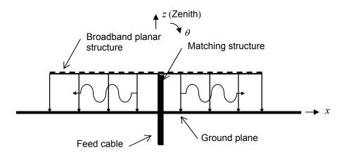
Figure 1. Mode-0 SMM antenna in transmit operation.
