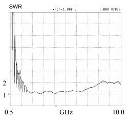
Figure 2. Measured SWR of mode-0 SMM antenna.
