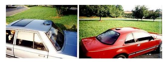
Figure 1. Multifunction SMM antennas mounted on rear rooftop of two passenger cars.
