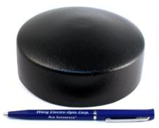
Fig. 1. Breadboard beamsteered array
