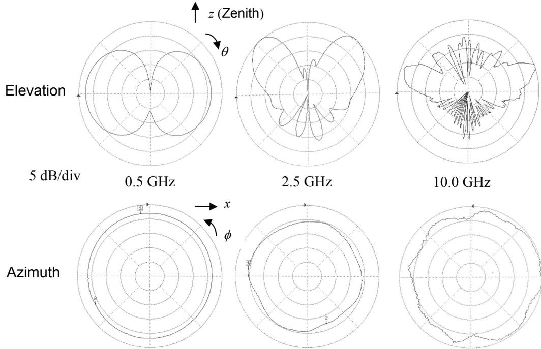
Figure 3. Representative azimuth and elevation patterns for the mode-0 SMM antenna.
