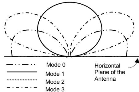
Fig. 2. Various patterns of the SMM antenna.
