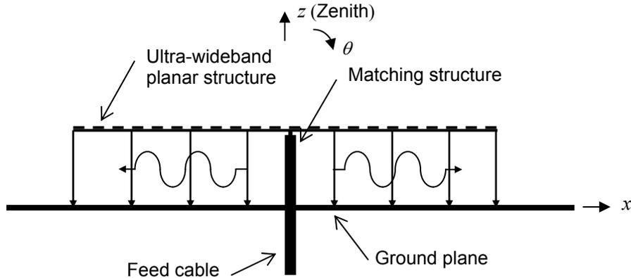
Fig. 1. Basic concept of the SMM antenna.
