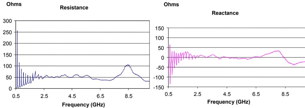
Fig. 4. Measured resistance and reactance of a mode-0 SMM antenna over 0.5-10.0 GHz.
