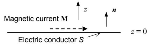
Fig. 3. Equivalent problem for exterior fields ( $z > 0$ ).
