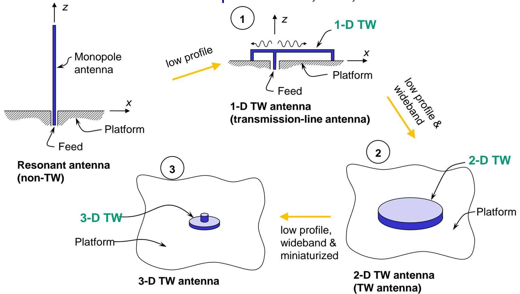
A broadband 2-D Traveling Wave Antenna (TWA) has circumvented the Chu Limit on antenna gain-bandwidth (Wang paper PIERS 2005)
