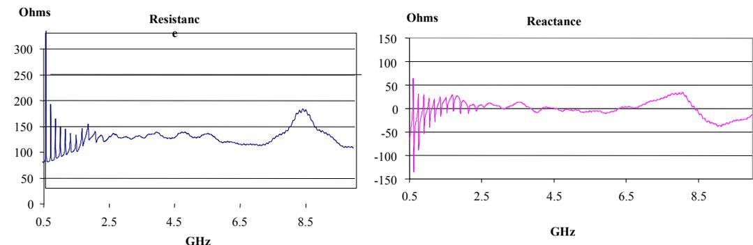
Fig. 2. Measured resistance and reactance of a TW antenna.
