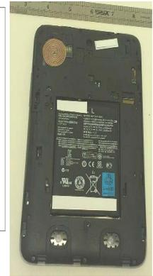
Fig. 4. AMUA in a mini-tablet with top cover removed.
