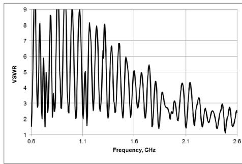
Fig. 3. Measured VSWR of the TW antenna
