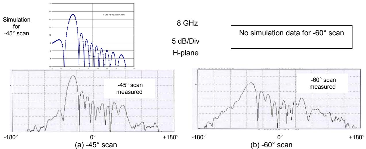
Fig. 2. Comparison of measured and simulated radiation patterns for wide scan to  $-45^\circ$  and  $-60^\circ$ .
