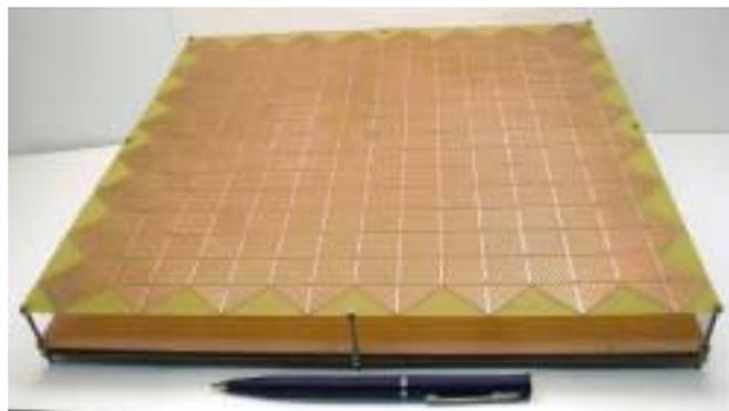
Figure 6: A planar array with 113 elements.
