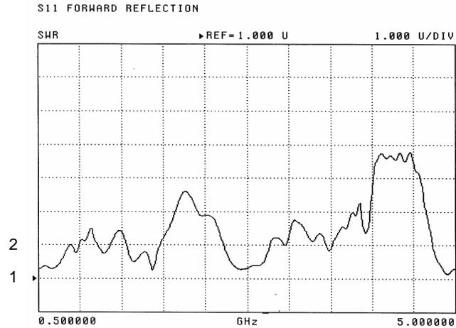
Figure 4: Measured SWR of the 5×5-element array of Figure 2.
