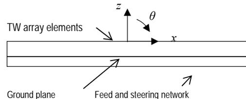
**Figure 1:** Cross-sectional view of a planar array.
