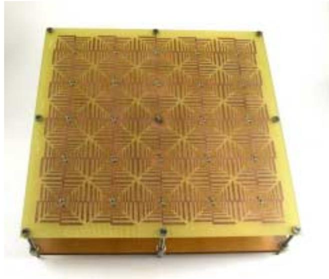
Figure 2: A planar array based on LP dipole elements.
