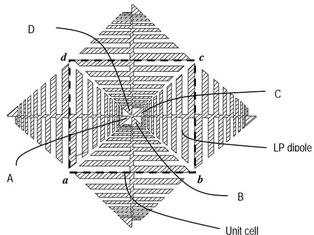
Figure 3: Unit cell of the planar array in Fig. 2.
