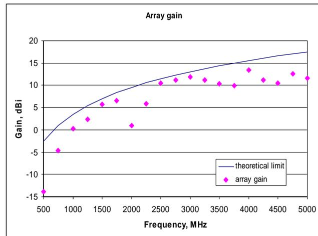
Figure 5: Antenna gain of the 5×5-element array of Figure 2.
