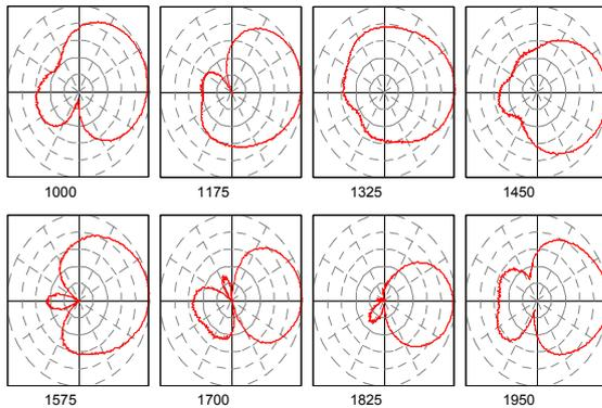
Figure 3: Measured azimuth radiation patterns.
