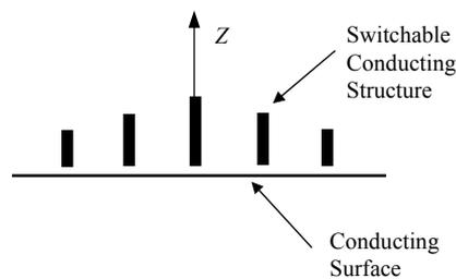
Figure 1: A broadband LP surface waveguide.
