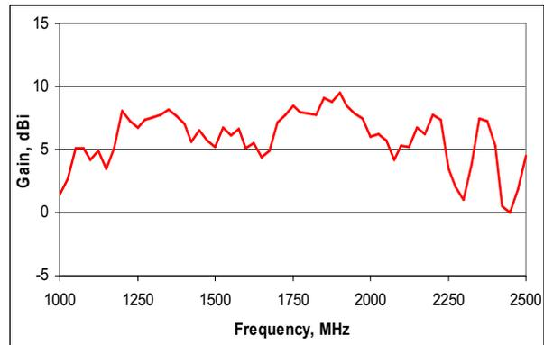
Figure 5: Measured peak elevation gain.
