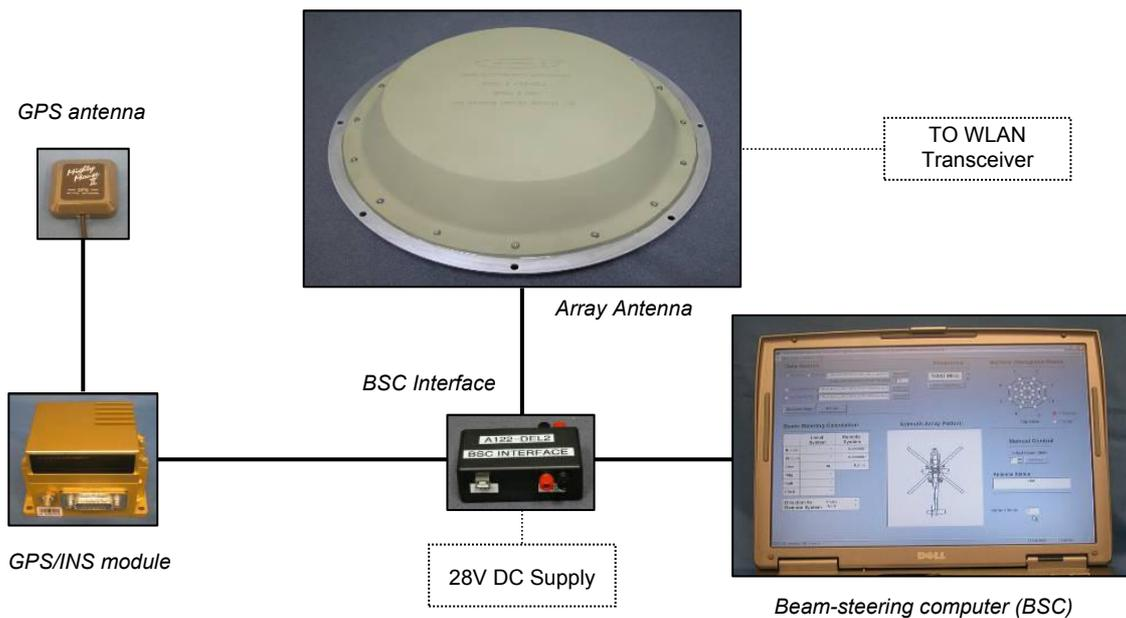
Figure 6: Assembly of a complete electronically-steered array.
