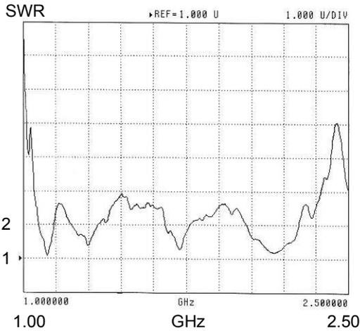
Figure 2: Measured SWR over 1–2.5 GHz.
