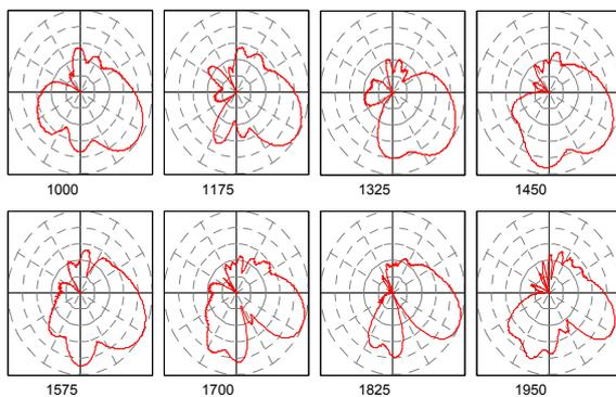
Figure 4: Measured elevation radiation patterns.
