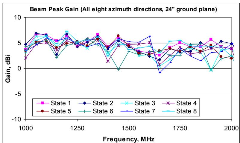
Figure 7: Measured antenna gain for electronically steered array.
