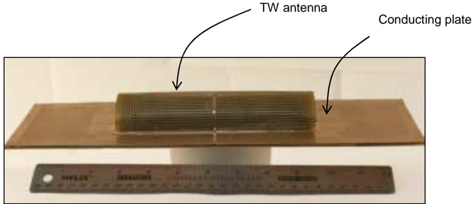
Figure 1. TW antenna on conducting platform.
