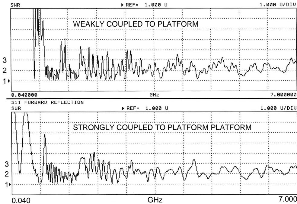
Figure 2. Comparison of measured SWR of TW antenna in Figure 1: TW antenna weakly coupled or strongly coupled to platform (upper and lower chart, respectively).
