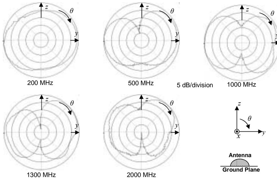
Figure 4. Typical measured elevation radiation patterns at  $\varphi = 90^\circ$  over 200 – 2000 MHz.
