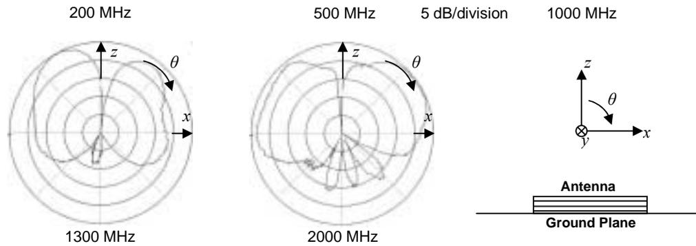
Figure 3. Typical measured elevation radiation patterns at  $\varphi = 0^\circ$  over 200 – 2000 MHz.
