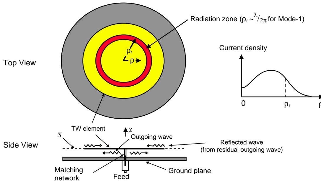
Figure 1. The planar TW antenna.
