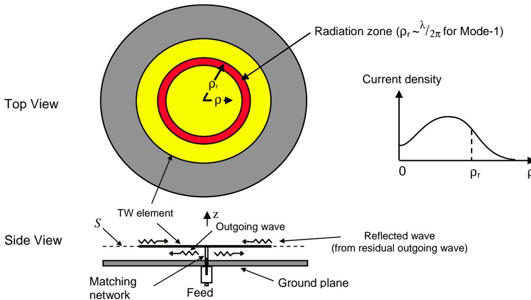
Figure 1. The planar TW antenna.
