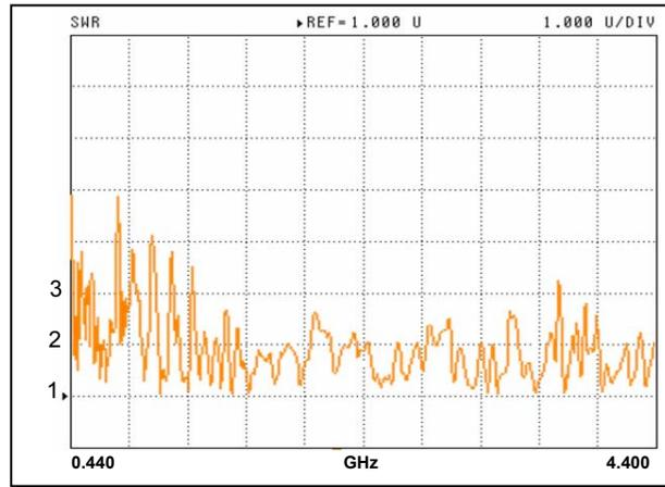
Fig. 2. Measured SWR over 0.44-4.40 GHz.
