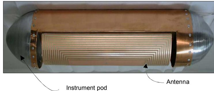
Fig. 1. Antenna on pod.
