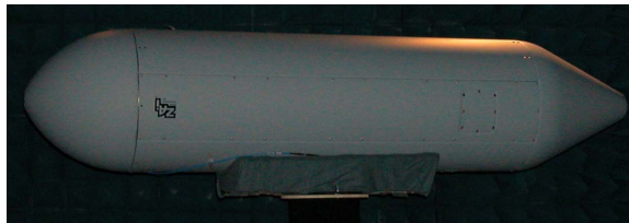
Fig. 2. Pod with antenna installed inside.
