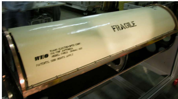
Fig. 1. Antenna on partially assembled pod.
