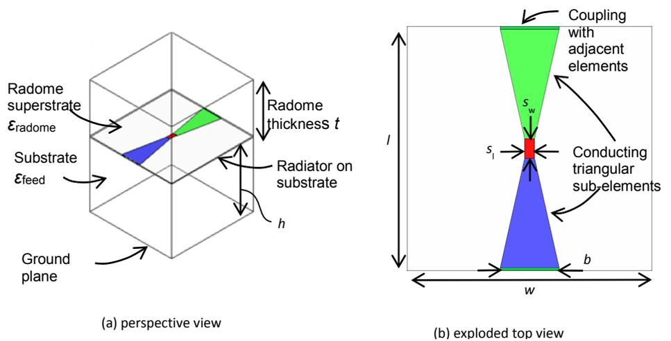
Fig. 1. Unit cell of the planar array with planar bowtie radiator.
