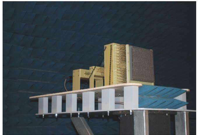
Fig. 5. A TWAA with three banks of TTD BSN being measured in WEO anechoic chamber.
